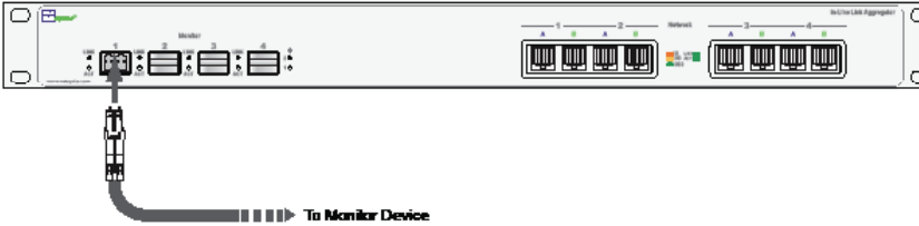
Figure 6: Connecting to Monitoring Devices using SFP modular connectors
